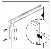
Fix the handle on the opposite side, insert the plastic plugs into the holes left open that can be found in the instruction for use bag.
